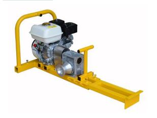
A lightweight capstan winch, designed for use over manholes, for simple cable pulling and cable recovery, powered by a 5HP Honda Engine through a right angle gearbox, the pulling capacity is 1000kg using a 12mm diameter rope (recommended) via a 100mm diameter aluminium Diablo capstan at a rope speed of 18m per minute.
